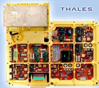
DC-DC converter and the USO fixed on
