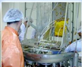
Preparation of SH characterisation in Thermal Vacuum. During SH AIV in CNES.
