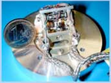
piezoelectric mechanism for laser beam intensity balance
